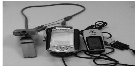
Fig. 9 Prototype node with video camera and GPS receiver attached.
