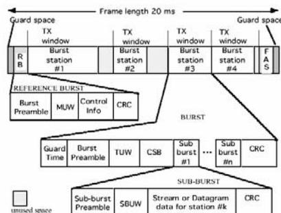
Fig. 3. Frame, Burst and Sub-burst Formats
