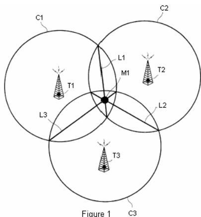
Figure3.3 illustrates a typical TOA method for locating a mobile telephone.
