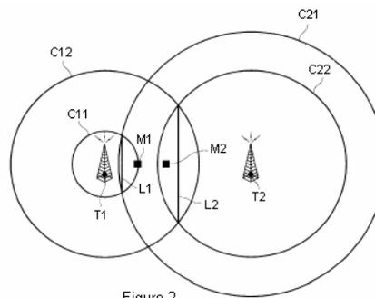
Figure3.4, illustrates the TDOA method of locating a mobile telephone.
