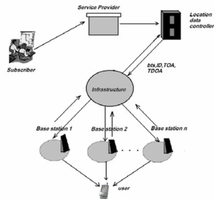
Fig 2.1 Architecture of a general Geolocation system
