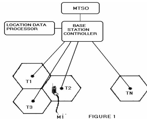
**Fig 1 Configuration of a typical mobile telecommunication network.**
