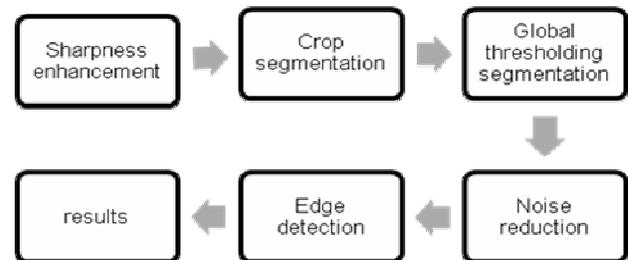
Fig2. Image processing algorithm flow
