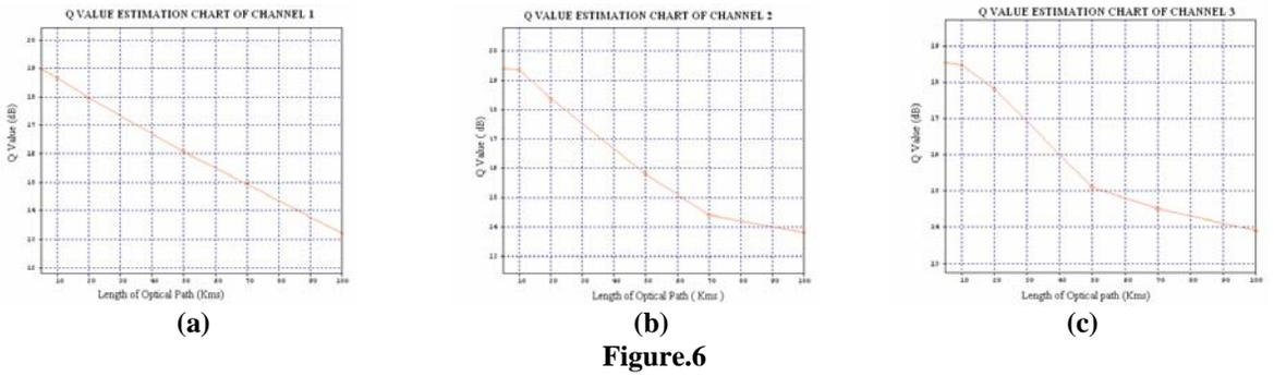
**Q value estimation chart (External Intensity Modulation) with (a) Channel 1 (b) Channel 2 (c) Channel 3**
