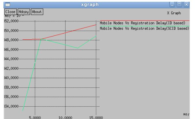
Fig. 3 Registration delay for various number of nodes
