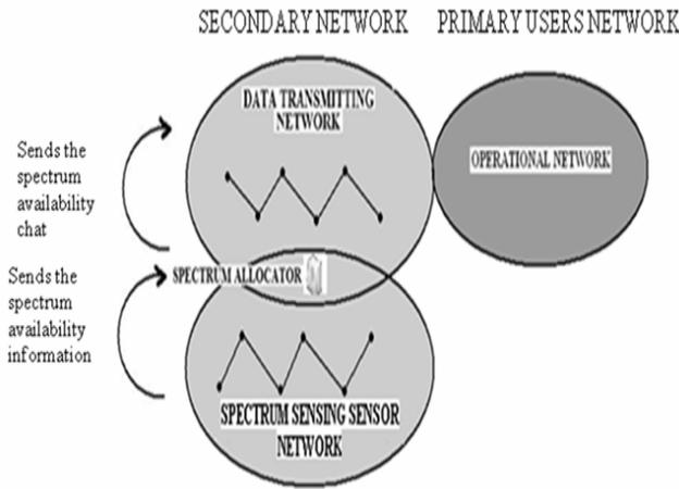
Figure 1. Proposed network architecture of cognitive wireless sensor network
