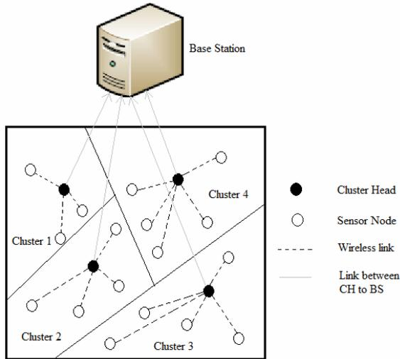
Fig 2: Basic CH Communication in DSC
