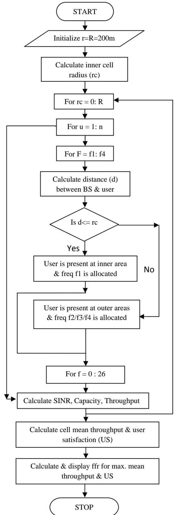
**Figure 3: Mechanism Flow**
