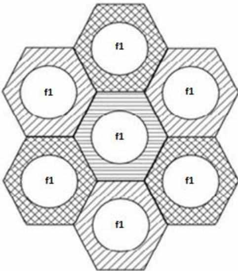
Figure 2: System topology using FFR scheme
