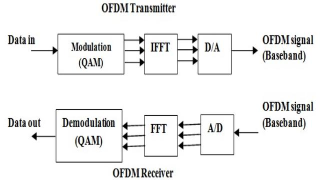
Figure 3: Block diagram of OFDM Transmitter and Receiver
