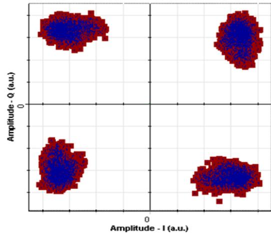
Figure 10: Constellation diagram RF-OFDM Receiver
