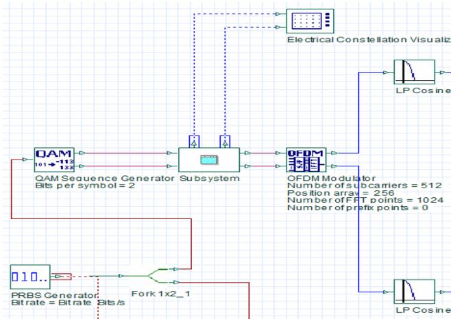
Figure 5: RF-OFDM Transmitter
