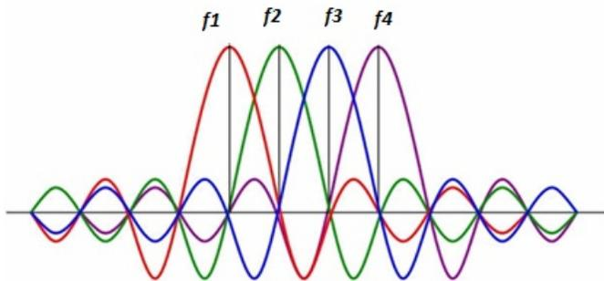
Figure 2: OFDM Spectrum
