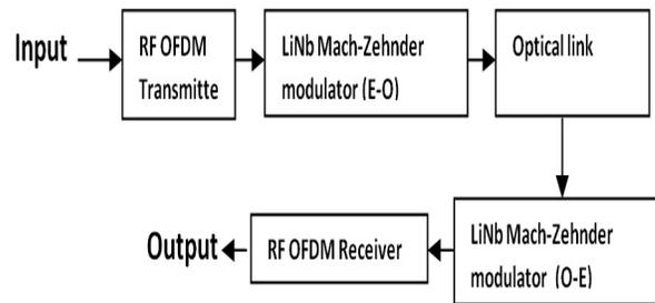
Figure 4: OFDM-RoF system model
