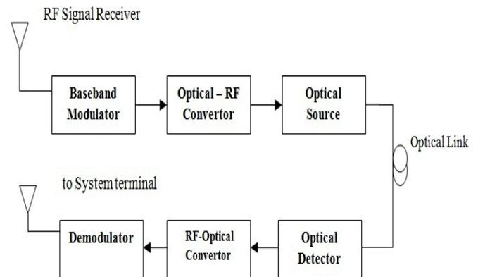
Figure 1: Block diagram of Radio over Fiber
