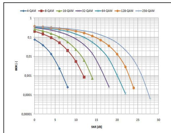
Figure 3. Measured BER dependency on SNR [8]
