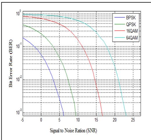
Figure 2. Simulation BER vs. SNR [6]
