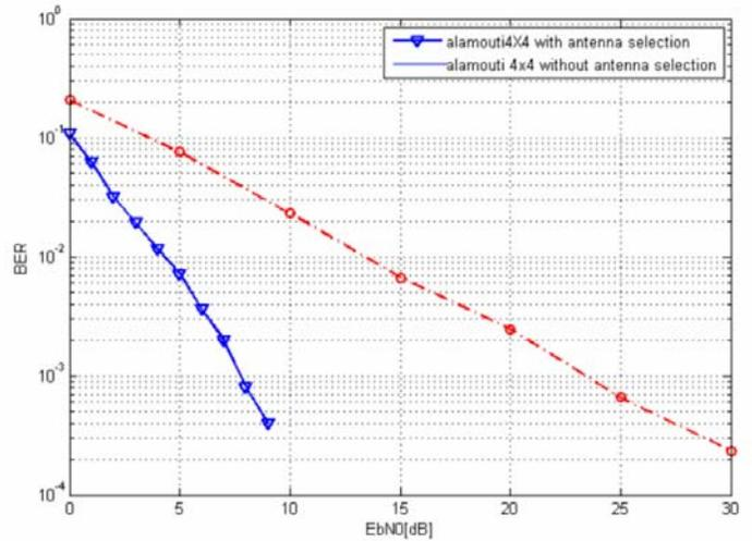
Figure 5. Error Performance for RAYLEIGH channel and BPSK modulation scheme
