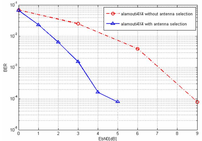
Figure 7. Error Performance for RICIAN channel and QPSK modulation scheme
