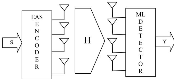
Figure 1. Block-Diagram representation of Extended Alamouti Scheme
