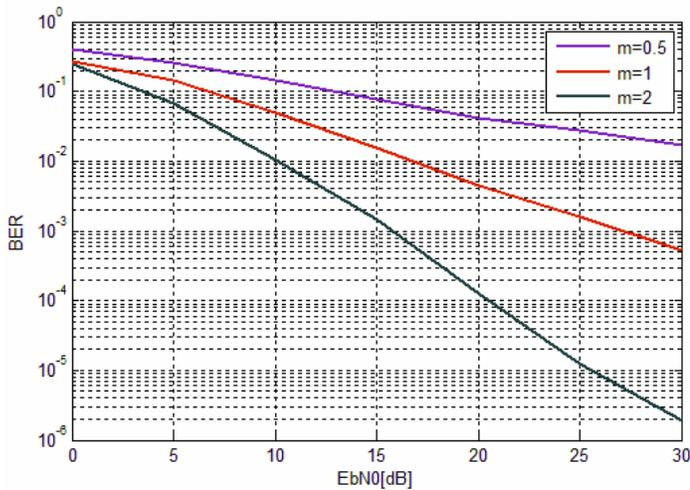
Figure 10. Error performance for NAKAGAMI channel and QPSK modulation scheme
