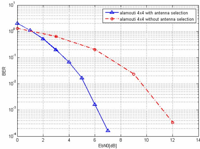
Figure 8. Error Performance for Rician channel and QPSK modulation scheme
