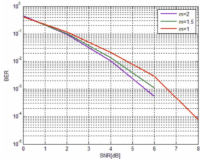
Figure 12. Error performance for NAKAGAMI channel and QPSK modulation scheme
