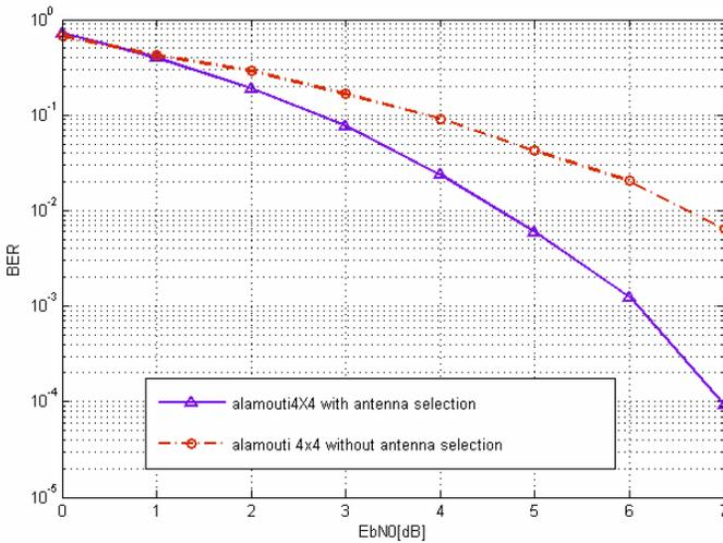
Figure 4. Error Performance for AWGN channel and QPSK modulation scheme
