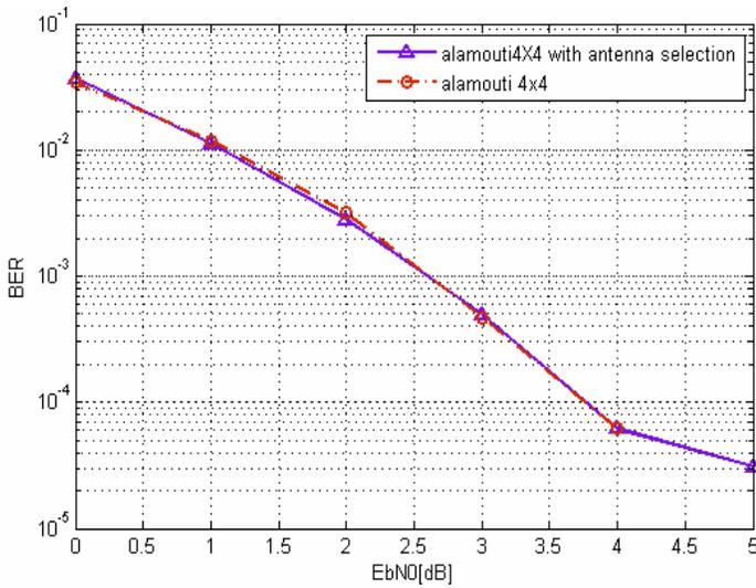
Figure 3. Error Performance for AWGN channel and BPSK modulation scheme
