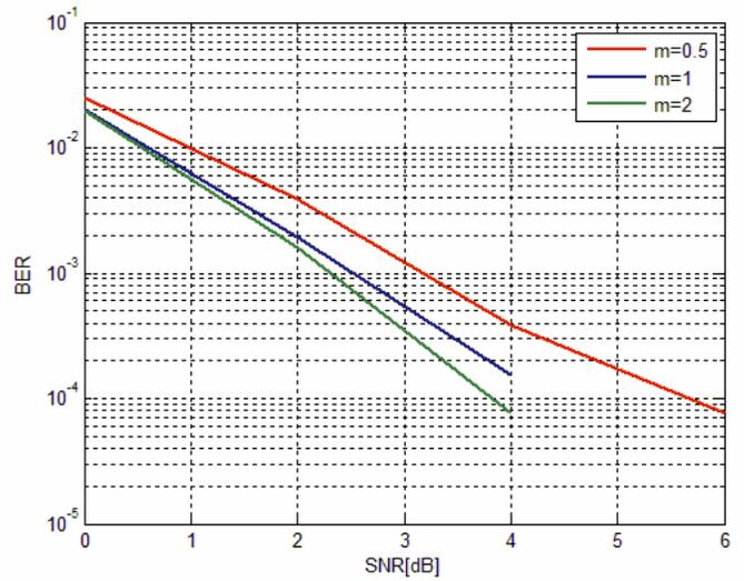
Figure 11. Error performance for NAKAGAMI channel and BPSK modulation scheme
