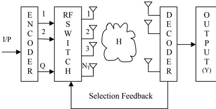
Figure 2. Block Diagram representation of TAS
