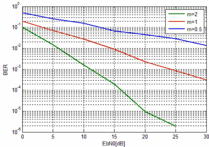
Figure 9. Error performance for NAKAGAMI channel and BPSK modulation scheme
