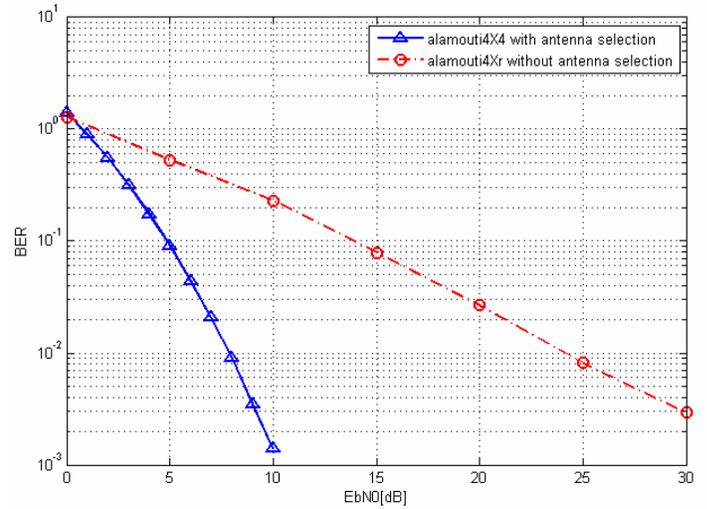
Figure 6. Error Performance for RAYLEIGH channel and QPSK modulation scheme
