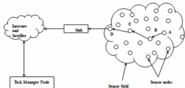
Figure1 Sensor nodes scattered in a sensor field
