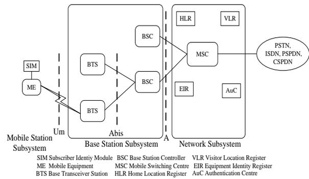
Figure 1: A GSM Architecture
