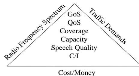
Figure 2: Inputs to cell planning
