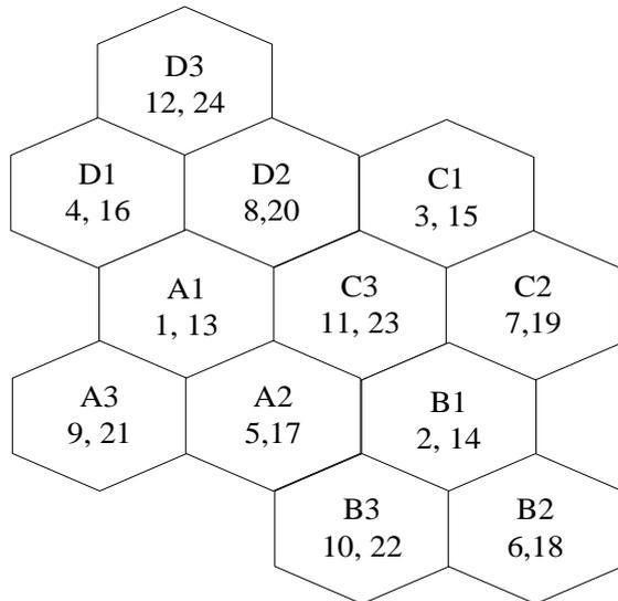
Figure 3: 4/12 cell cluster for a 24 group of channels
