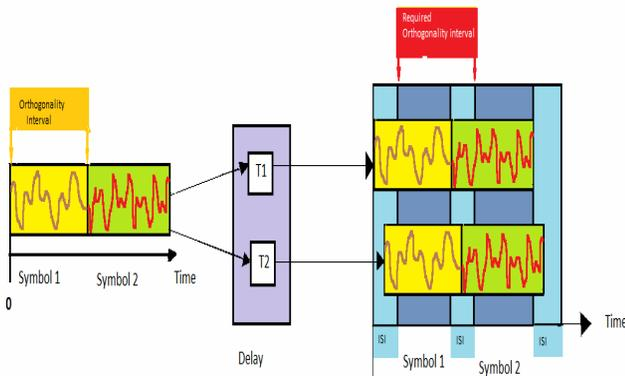
Fig.3. OFDM Transmission Without Cyclic Prefix
