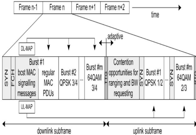
Fig.1. Frame Structure of IEEE 802.16
