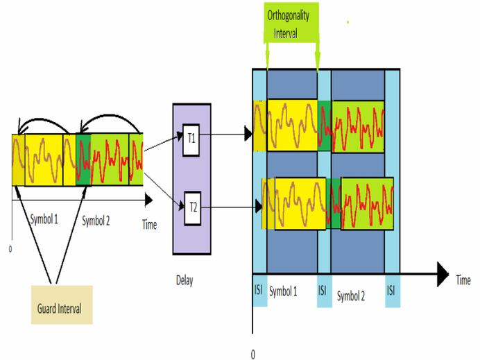
Fig.4. OFDM Transmission With Cyclic Prefix
