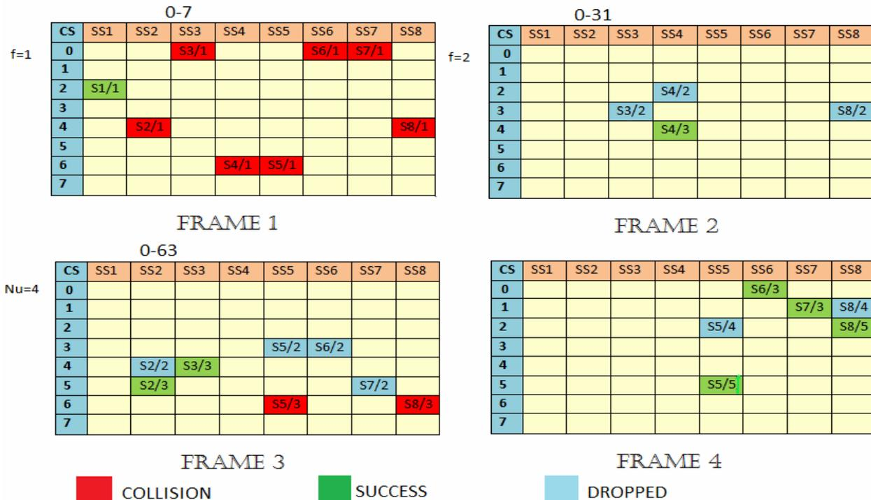
Fig.2. Frame Analysis of BWR Mechanism with Circularity =2
