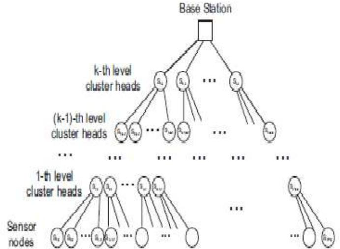
Figure 4 . Hierarchical structure of the sensor network
