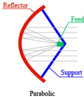
Fig 2: Parabolic Reflector
