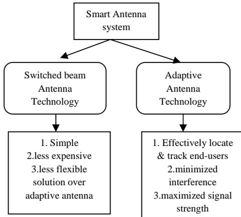
Figure 1: Antenna Comparison
