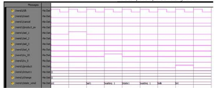
Fig 5: Simulation waveform showing selection of milk pouch
