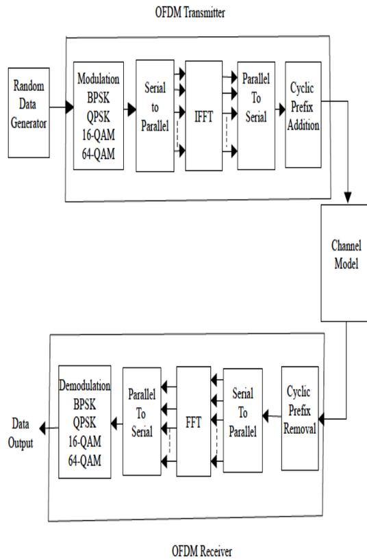
Figure 3: OFDM Transceiver
