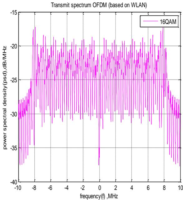
Figure 6: Plot of Power Spectral Density against frequency for 16-QAM in WLAN
