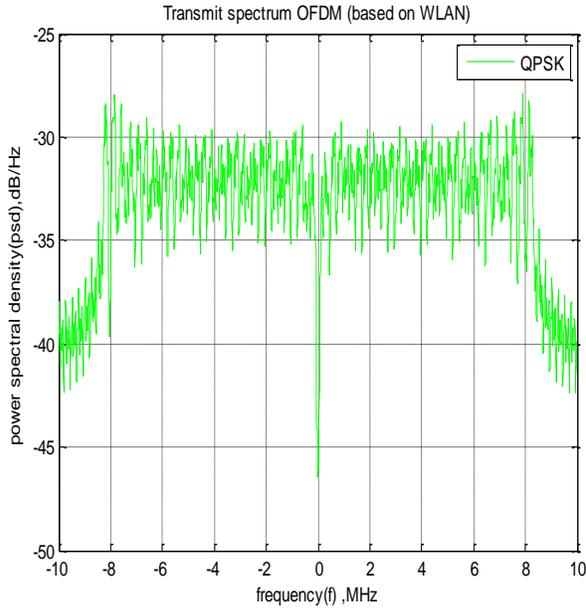
Figure 5: Plot of Power Spectral Density against frequency for QPSK-WLAN
