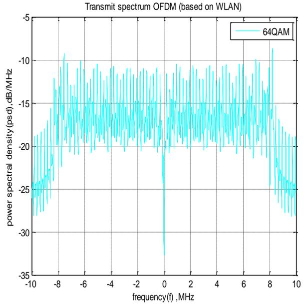
Figure 7: Plot of Power Spectral Density against frequency for 64-QAM in WLAN
