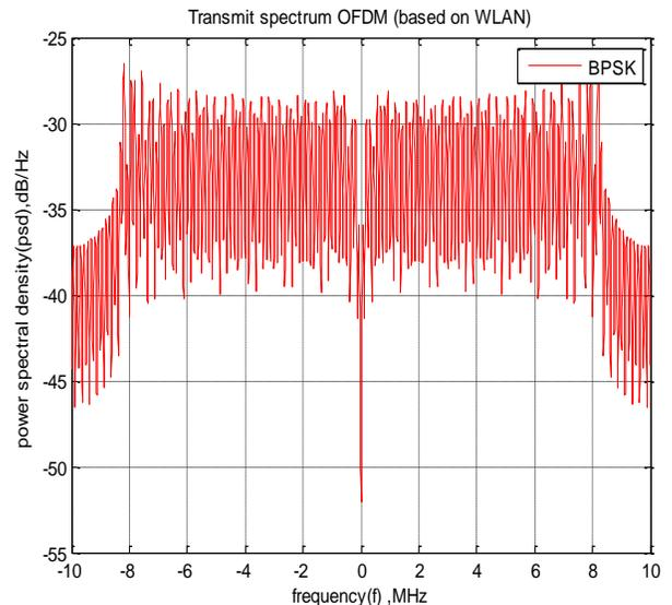
**Figure 4: Plot of Power Spectral Density against frequency for BPSK-WLAN**
