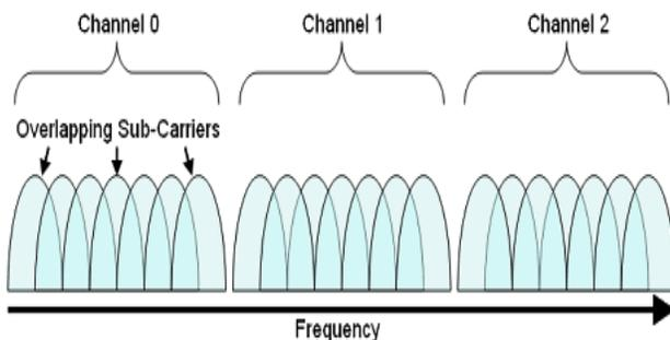
**Figure 2: Spectral efficiency of OFDM [5]**
