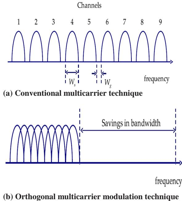
**Figure 1: Concept of the OFDM signal: (a) conventional multicarrier technique, and (b) orthogonal multicarrier modulation technique[7].**
