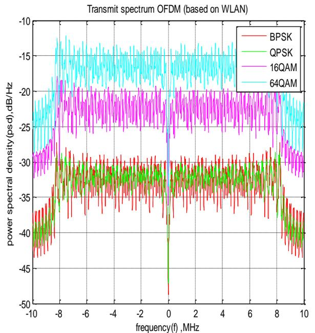
Figure 8: Transmit power spectrum for all digital modulation techniques in WLAN
