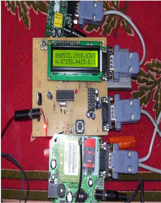
Fig 7 Complete hardware setup
