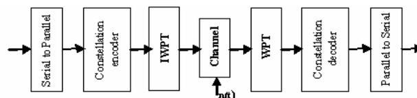
Figure 1. Block Diagram of WPM System
