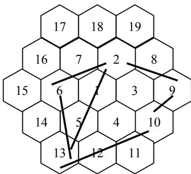
Figure. 1 Base Network (cellular network showing active calls from pairs of mobile users)
