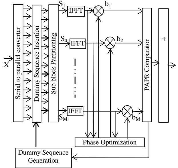
Figure.1. Block Diagram of Proposed CSI-PTS Technique
