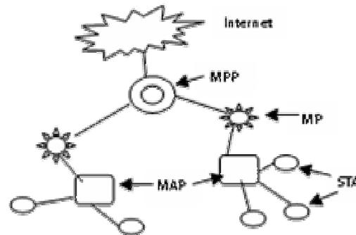
Figure 1. Example Wireless Mesh Network
