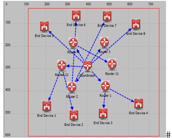
Fig2. ZigBee Tree network
