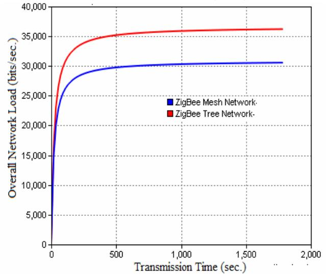
**Fig 6. Overall Network Load w.r.t Simulation Time**
