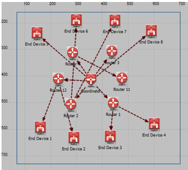
**Fig4. ZigBee Mesh network after Routing**
