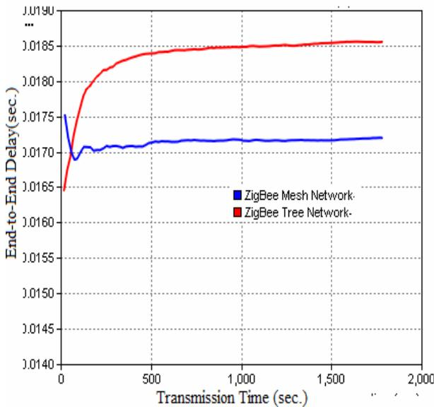
**Fig 5: End-to-End w.r.t Simulation Time**
