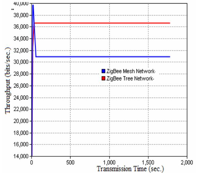
**Fig7. Overall Throughput w.r.t Simulation Time**
