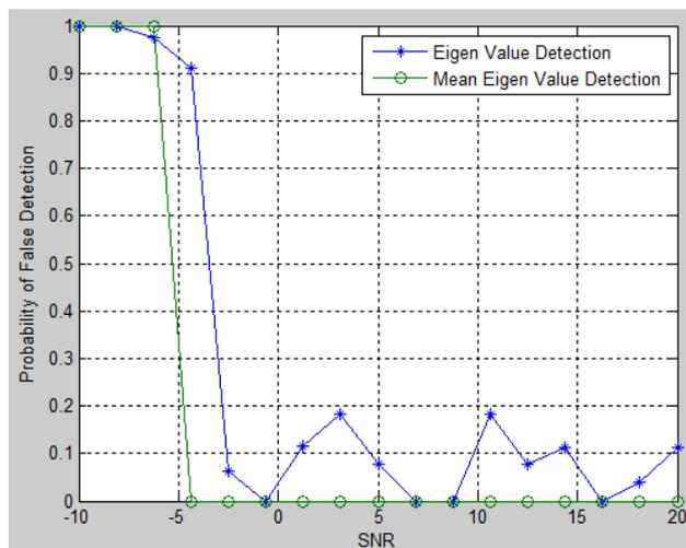
Figure 3: Probability of False Detection vs. SNR for all Detection Methods
