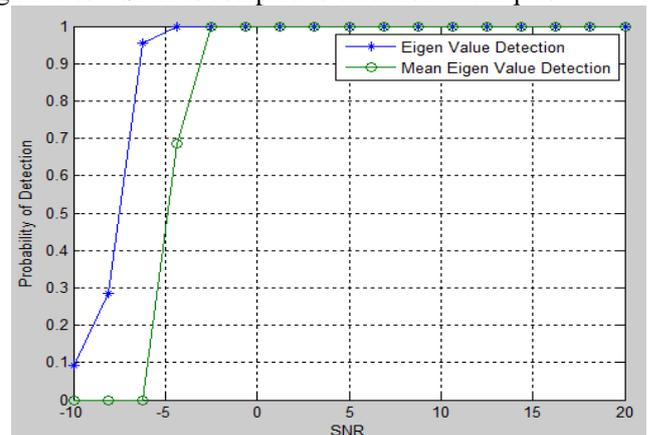
Figure 1: Probability of Detection vs. SNR for all Detection Methods
