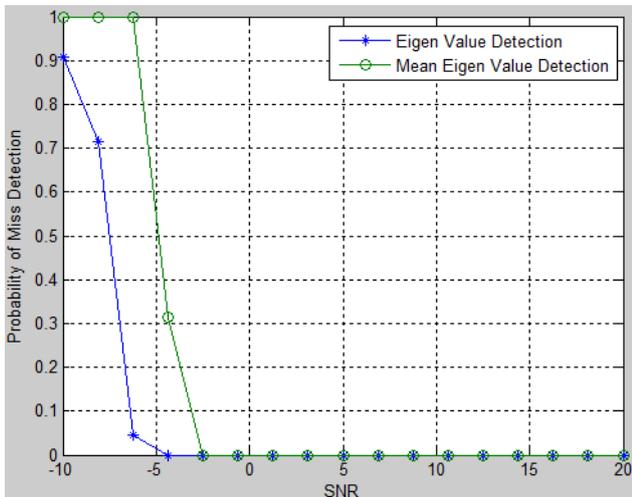
Figure 2: Probability of Miss Detection vs. SNR for all Detection Methods
