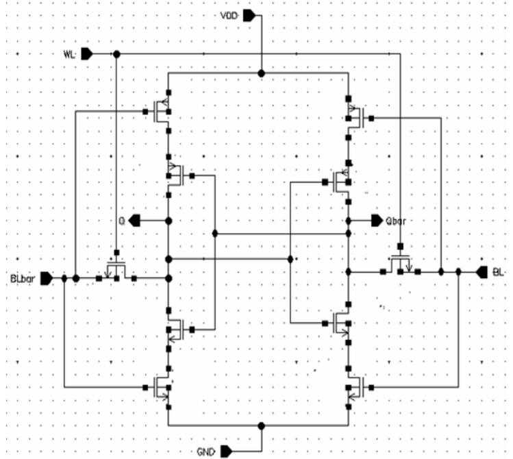
Fig.2: Schematic of Force Stack SRAM Cell
