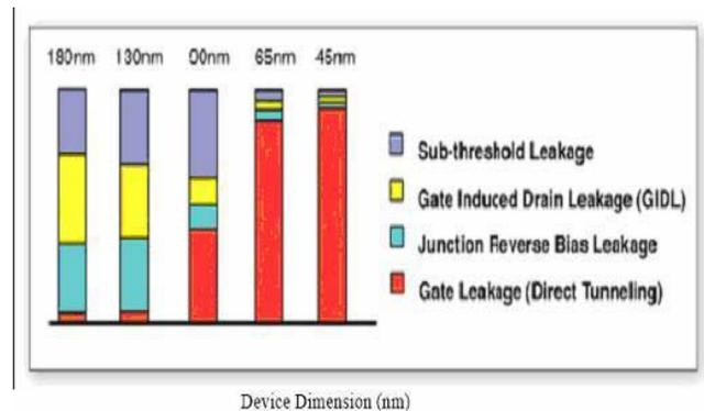
Fig.1. Power Dissipated in various Technology
