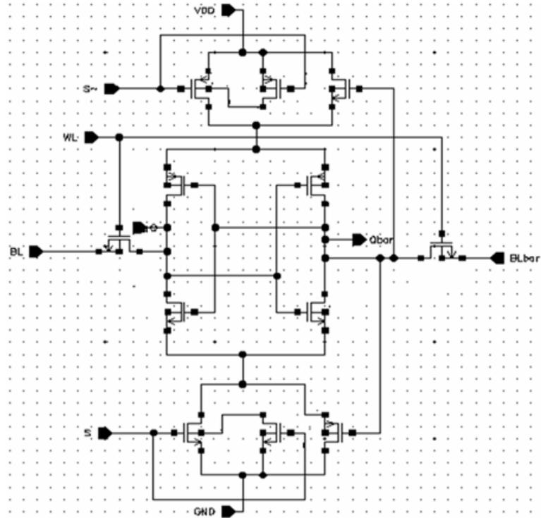
Fig.4 Schematic of Variable Body Biasing SRAM Cell
