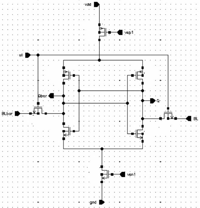
Fig.1. Schematic of Sleep Transistor SRAM Cell
