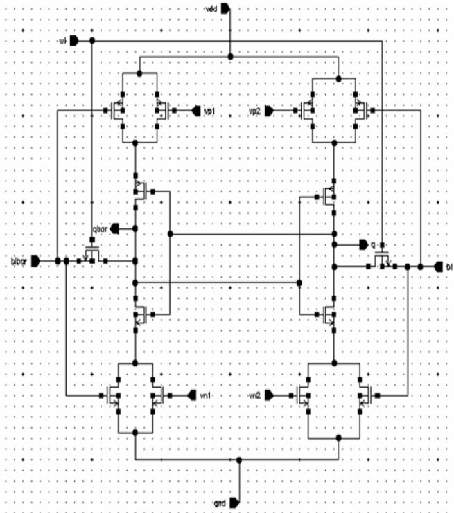
Fig.3. Schematic of Sleep Stack SRAM Cell
