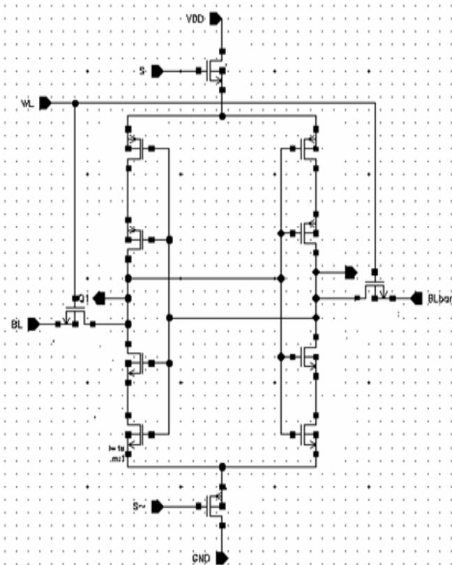
Fig.5. Schematic of Force Sleep SRAM Cell
