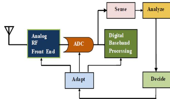
Figure 3. Cognitive radio adds Sense, decide and Adapt blocks to the SDR.
