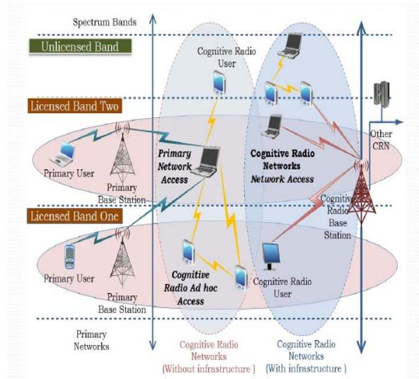
Figure 4: Cognitive Radio Architecture
