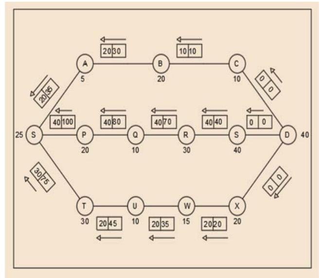
Fig.4. the Propagation of RREP packets
