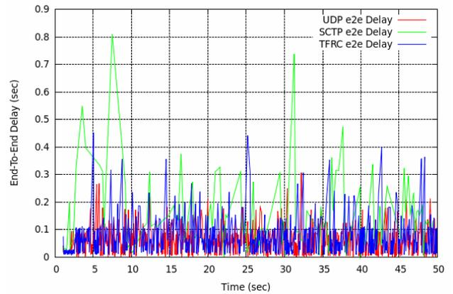
Fig. 5. End-to-End for VoIP with G.726 codec
