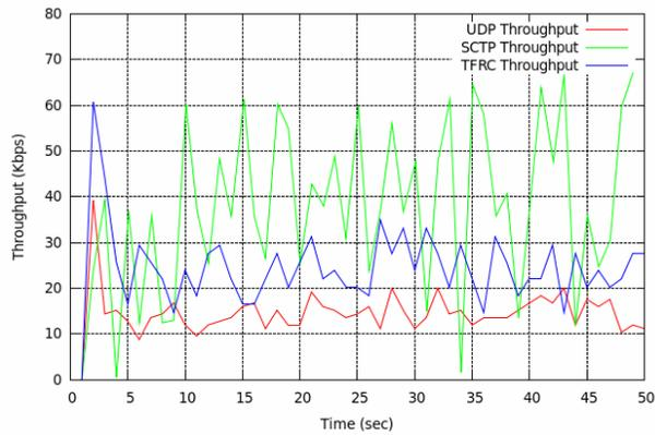
Fig. 3. Throughput for VoIP with G.726 codec
