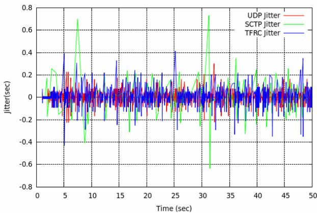
Fig. 7. Jitter for VoIP with G.726 codec
