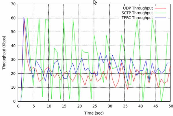
Fig. 2. Throughput for VoIP with G.711 codec
