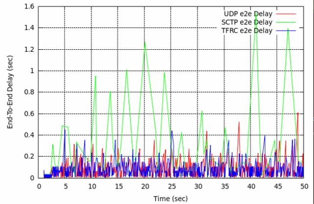
Fig. 4. End-to-End for VoIP with G.711 codec
