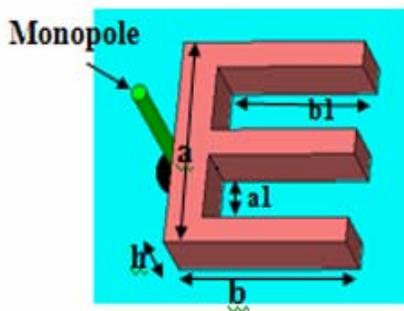
Figure 1. Geometry of E shaped monopole DRA
