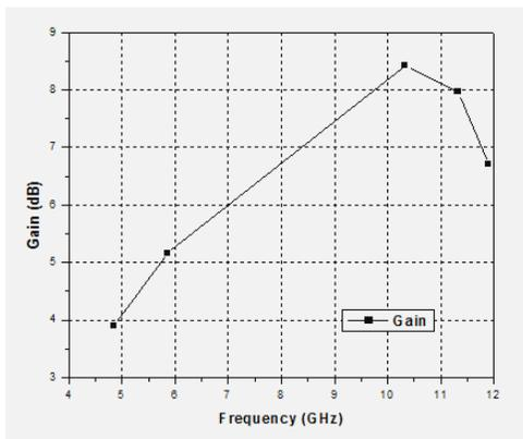
Figure 9. gain v/s frequency plot of proposed antenna
