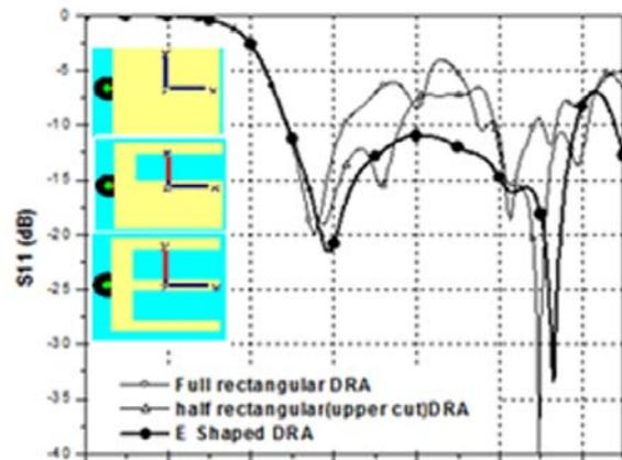
Figure 2. Simulated return loss characteristics of three different designs shown in inset
