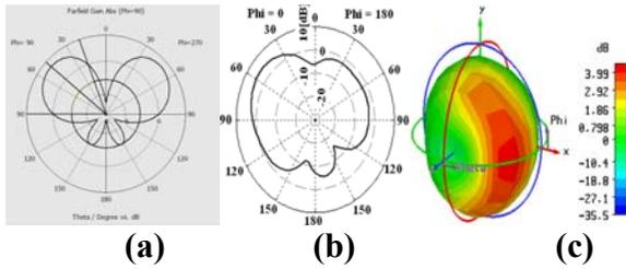
Figure 7. Simulated radiation pattern (a) xz plane (b) yz plane (c) 3D radiation Pattern at 5.8556 GHz.
