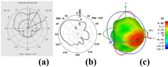
Figure 8. Simulated radiation pattern (a) xz plane (b) yz plane (c) 3D radiation Pattern at 11.326GHz
