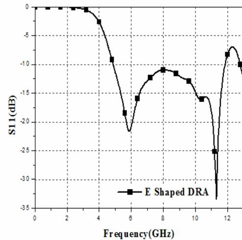
Figure 6. Return loss plot of E shaped DRA with monopole arrangement
