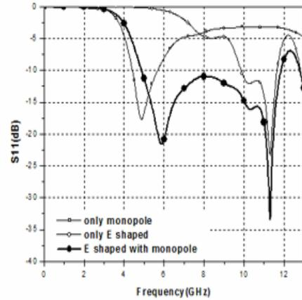
Figure 5. Simulated return loss plot of comparison of only monopole, only E shaped and E shaped with monopole arrangement
