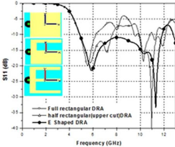
Figure 3. Simulated return loss versus frequency of monopole-fed DRA having variable probe pin length as fig.1
