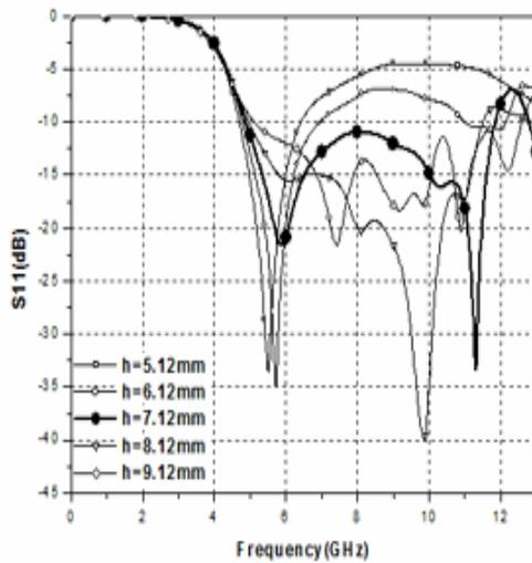
Figure 4. Simulated return loss versus frequency of monopole-fed DRA having Different height of DRA
