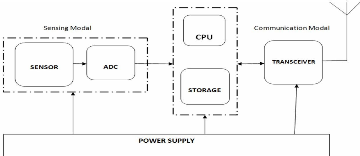
**Figure1: Architecture of wireless underground sensor node**
