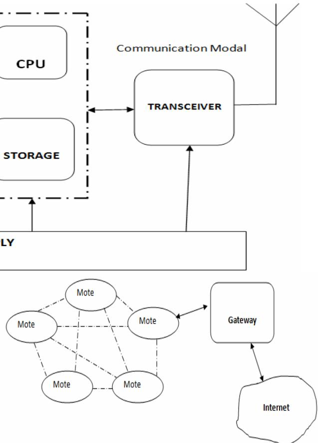
**FIGURE2: COMMUNICATION BETWEEN MOTE AND GATEWAY**
