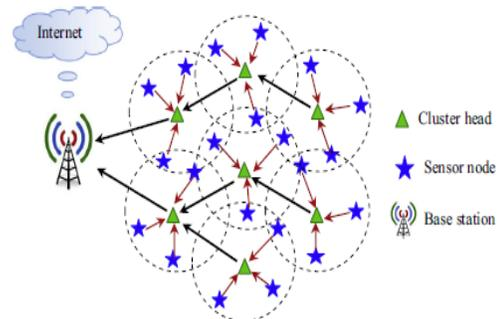
Fig. 1 Model of wireless sensor network
