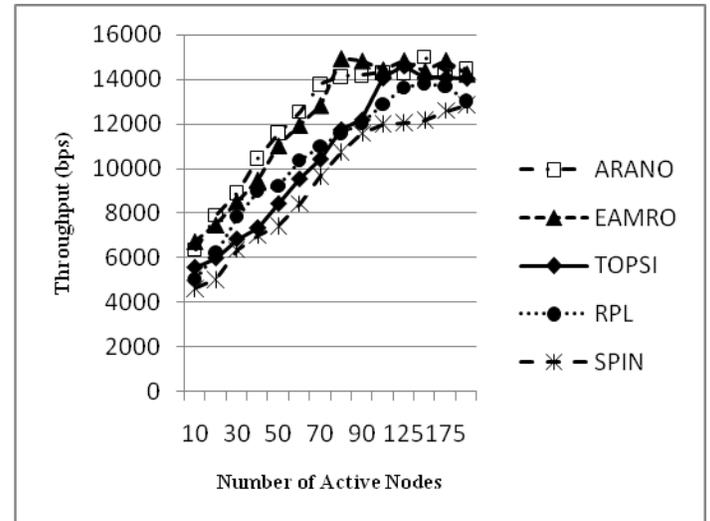
Fig. 5Throughput Observed in ARANO over Traditional Route Approaches
