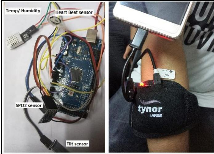
Fig. 4IoT Client Module and ARANO Module with Support for Routing, QoS and Data Collection
