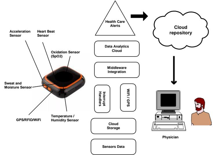
Fig. 3 Architecture and Prototype Module of ARANO
